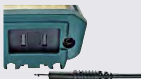
Connection for external power pack and continuous, battery-free power supply
