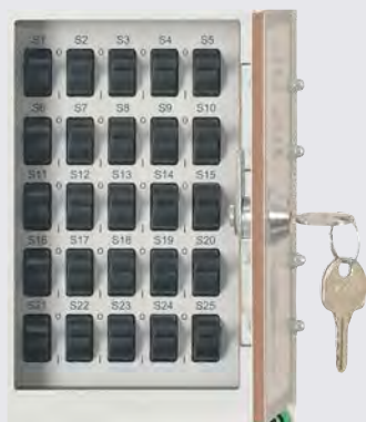
Error Simulator with 25 Error Options via Switches
