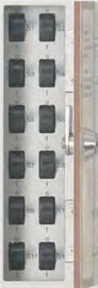
Error Simulator with 12 Error Options via Switches
